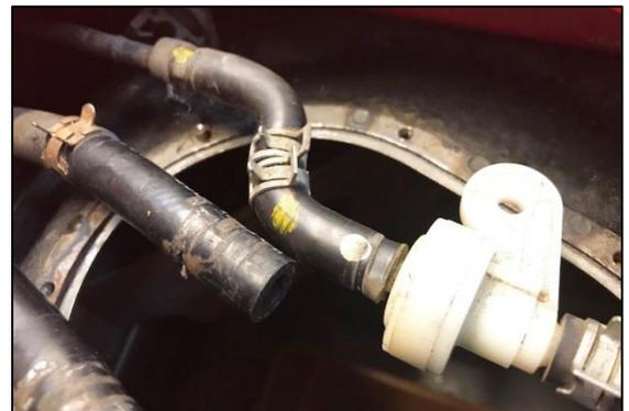
43. Rotate the rubber vent hose 180 degrees and secure with the spring clamps, as pictured.
