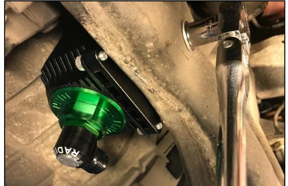
8. Find the long 8AN PTFE hose in the kit and attach the end with the 45 degree non-swiveling hose end to the fuel filter outlet (green side) as shown in the picture. Route the hose along the subframe to the area by the OEM fuel lines. Once the hose is situated, tighten the hose end to the fuel filter outlet using a 7/8" wrench.
