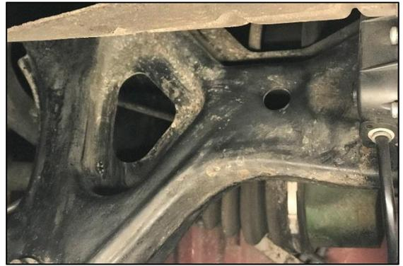
7. Install the fuel filter assembly with the black end of the filter upwards. Make sure the hose from Step 5 is routed up toward the fuel pump hanger and passes in front of the rear sway bar. Slide the long M8 bolt on the filter mount through the hole in rear subframe. Install the M8 washer and locking nut. Use a 13mm socket wrench, but do not torque the nut yet.
