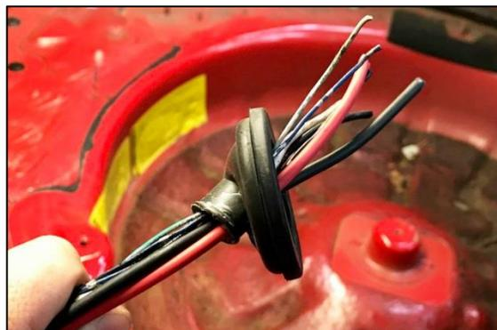
61. Reattach the rubber grommet to the OEM fuel tank access cover. Allow ample slack for terminating the wires in the following steps.
