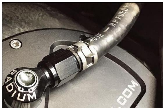
64. Turn the ignition key to the ON position to pressurize the fuel system. Confirm the new fuel pump(s) are properly operating. Check for leaks. If no leaks are found, start the vehicle.
