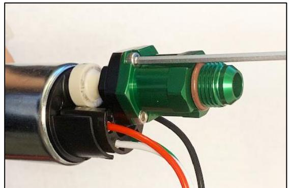
24. After tightening all bolts evenly, inspect the internal side of the green fitting. When installed properly, the plunger should be slightly sticking out of the center hole at rest, as shown.
