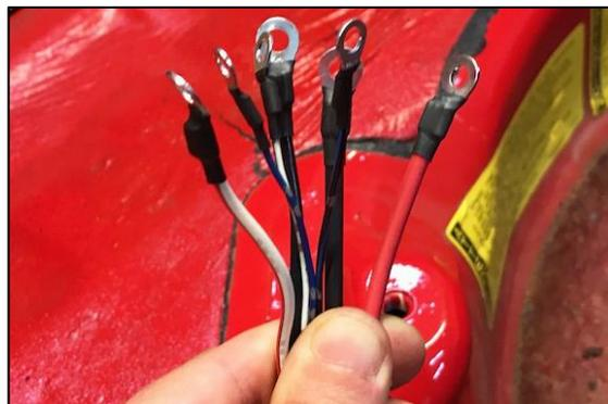
63. Referencing the chart, secure all ring terminal connections to the electrical studs using the provided acorn nuts and an 8mm socket wrench. Do NOT overtighten.
