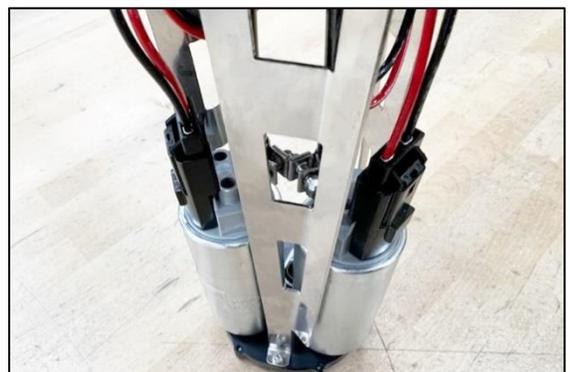
34. Before fully seating the FST canister to the top plate, correctly position the electrical wires. The black sensor ground wire should NOT enter the FST canister. The black connector with the green and white wires will be used for the fuel level/low fuel sensor.
