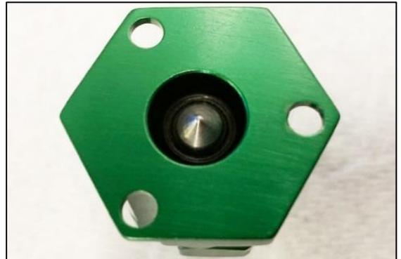
23. Apply a high-strength thread locking compound to the threads on the 3 included bolts. Line up the green fitting holes to the black fitting threads. Use a 2.5mm Allen wrench.
