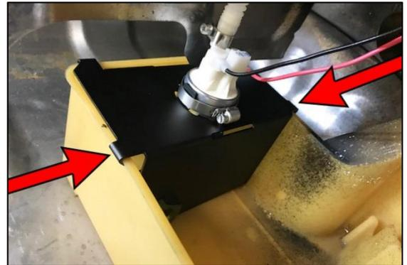
47. During acceleration, the check ball will open supplying the lift pump with ample fuel located inside the OEM sub tank as shown.
