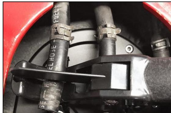
66. Push the OEM hoses onto the barb and secure with the OEM spring clamps, as shown.
