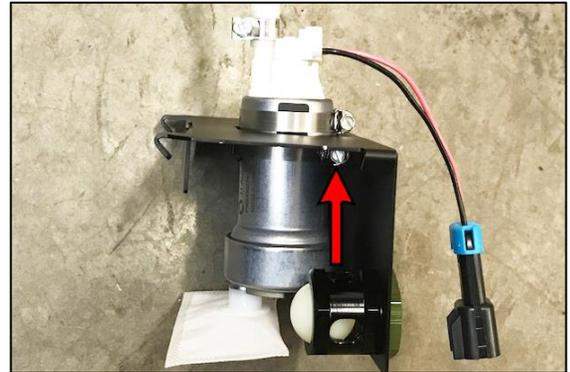
38. Find the OEM fuel level sender float/temperature sensor probe assembly.
