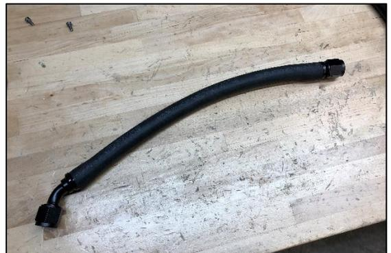
5. Attach the 45 degree hose end to the fuel filter inlet (black end). Tighten using a 7/8" wrench. It is a good idea to hold the swiveling fitting with an adjustable wrench while tightening the hose end.
