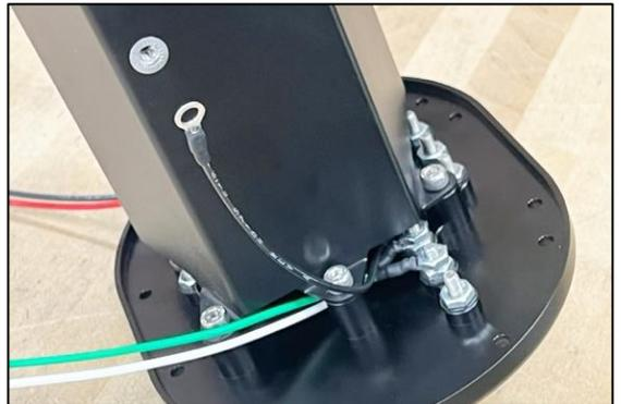
9. Using a 4mm Allen wrench, remove the 4 bolts that attach the FST canister to the top hat. Separate the two parts, as shown.
