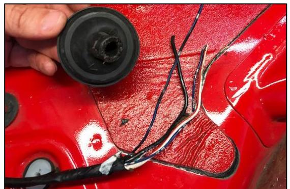
59. The OEM fuel pump power wiring will be reused for the lift pump. The OEM wiring does NOT need to be upgraded since the lift pump operates at very low pressure thus low current.
