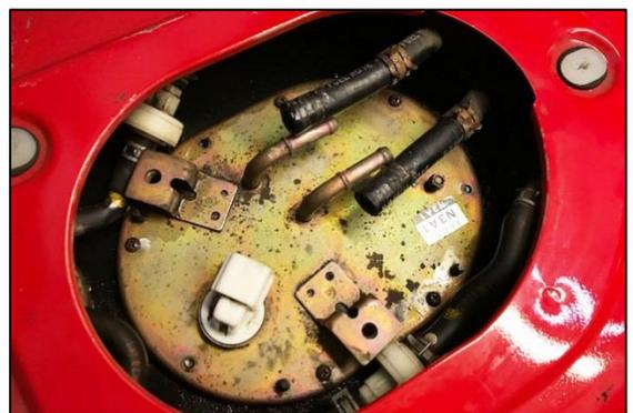
4. It is necessary to drain the tank to reduce fuel spills for an easier and safer installation.
