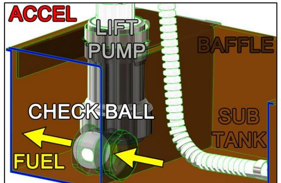
48. During deceleration, the check ball will close preventing fuel inside the OEM sub tank from escaping baffled area.
