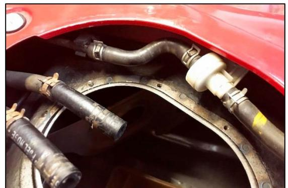
44. Plug in the 2-wire extension harness with the white connector to the lift pump. Lower the baffled lift pump assembly into the gas tank as shown.
