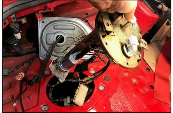
6. NOTE: If installing into a late model Mazda RX7 (FD), there will be a silver baffle on top of the internal sub tank, as shown. This metal plate must be removed. Both early and late model RX7s will benefit from the Radium Engineering baffle replacement in later steps.
