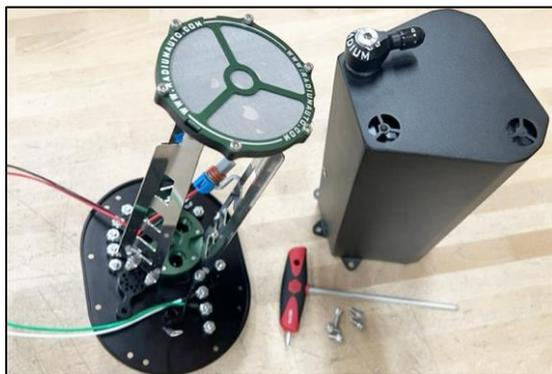
10. To remove the fuel pump mount, unscrew the 6 bolts shown using a 3/32" Allen wrench. Separate the parts, as shown.
