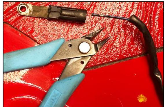
58. Unravel the electrical tape and remove the access cover rubber grommet from the wiring harness, as shown.
