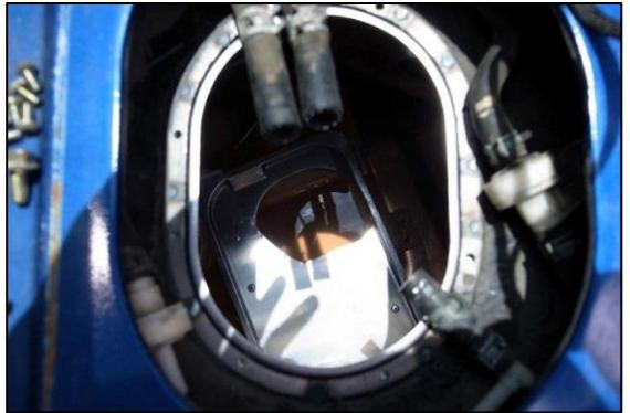
7. Only 2 parts will be reused from the OEM Mazda unit (gasket and sensors).
