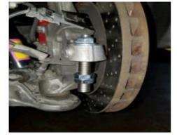
4. Remove the two jam nuts and install the spacers. The number of spacers needed depends on the amount of bumpsteer correction needed. Install the nylock nut (8) on the bottom and torque to 80 ft-lbs.
