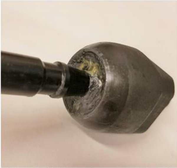
Figure 1: Factory packed grease in tie rod.
