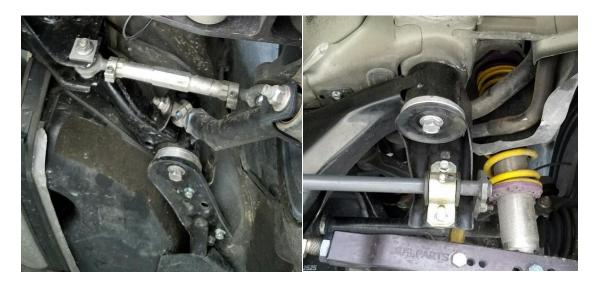
7. The supplied rubber isolators can be optionally installed between the chassis and the subframe bushing to help dampen some noise.
