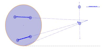
The following diagram shows what happens when you raise the subframe closer to the chassis. For this example, we are comparing what happens to the anti-squat when the ride height remains the same. When the subframe is raised, the rear "instant center" is raised as well, that moves point A up and increases anti-squat.
