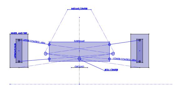
The following diagram shows the subframe raised closer towards the chassis (no more gap between subframe and chassis), and the ride height lowered the same amount. The roll center position is un-changed.
