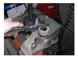
7. Measure the diameter of the new bushing and confirm that the new bushing is .001 - .003 inches (.025 - .076 mm) larger than the bore on the knuckle. If the tolerance is out of specification, please contact us for a replacement bushing.
