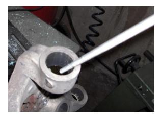
9. Lightly tap the new bushing into place to start, making sure the bushing is square against the bore.
