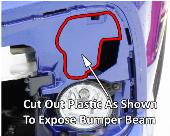
Remove Fog Light Cover and Locate Upper Holes On Bumper Beam
