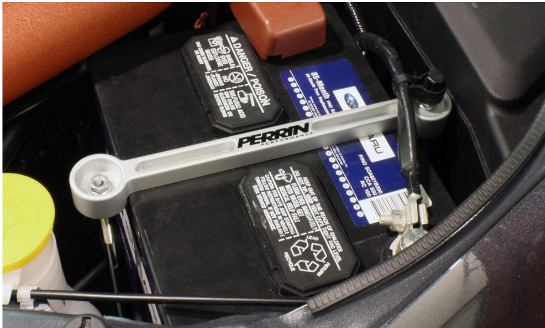
Above picture shows battery tie down on a 2008 WRX
