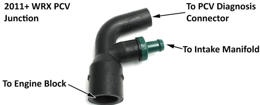
Picture above shows 2011-14 WRX PCV Junction with PCV diagnosis connector removed from upper hose.
