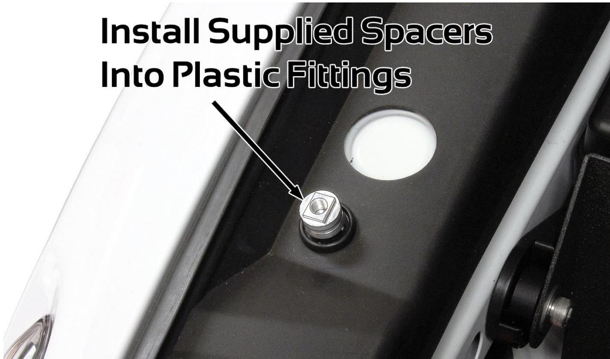
Above picture show the longer threaded push rivet installed into the center plastic fitting
