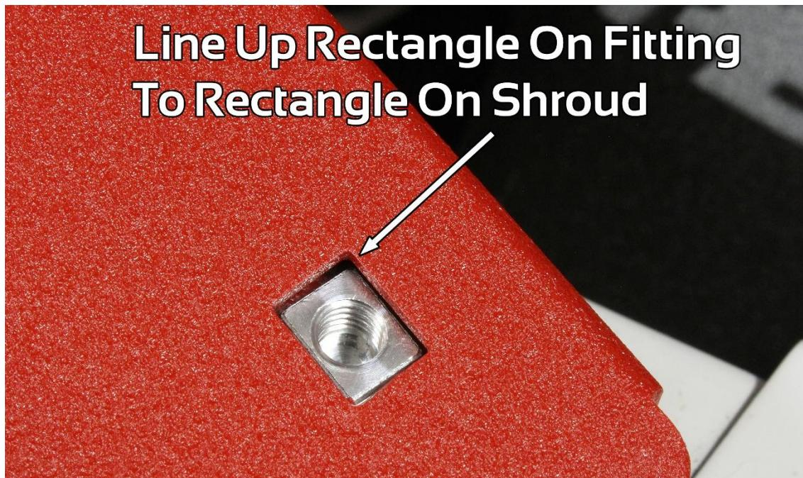
6. Install fender shrouds onto fittings and push down slightly to get the fittings to line up with the slots in fender shrouds. **NOTE: It is normal to have to compress the OEM rubber shroud down a bit to get them to line up.**
