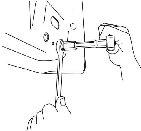
NOTE: Hold Rivet tool with wrench while loosening bolt.
