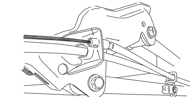
Attach brake cable guide to supplied Brake Cable Bracket (27) and mount bracket with supplied hardware. Reattach brake cable and readjust brake cable adjustment nut to original position.
