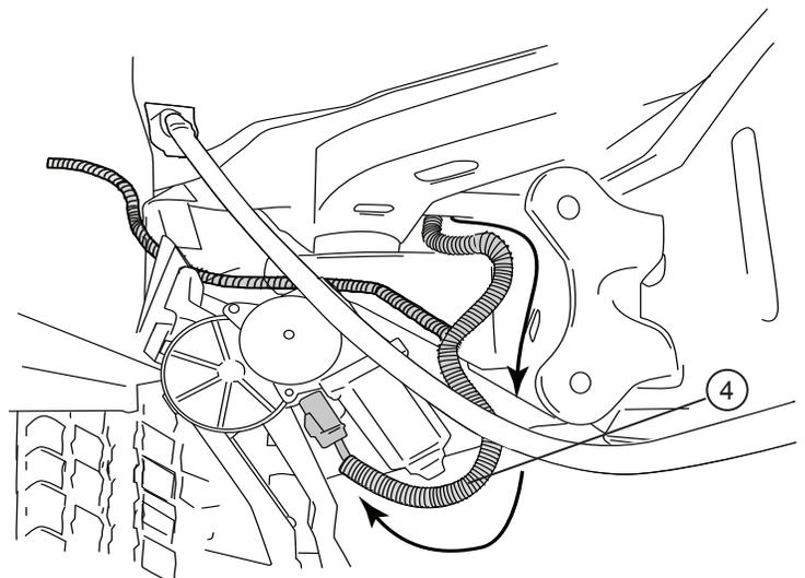
On Passenger Side, run Wire Harness leg down and along underside of the vehicle floor and frame to front Drive Linkage. Connect harness to motor and secure harness with tie wraps. Route remainder of wire harness towards rear linkage assembly for LED lights.
