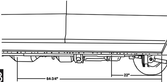
Drill a 9/32" hole through the pinch weld at marked locations. Deburr all holes. After drilling apply paint to holes to prevent rusting
