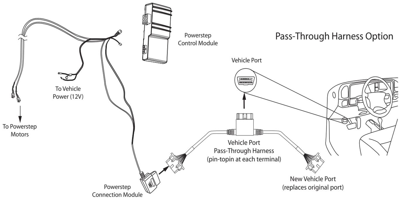
Route the two Wire Harness legs down over the wheel wells toward Motor Linkages, long leg across to the passenger side. Secure harness with tie wraps.
