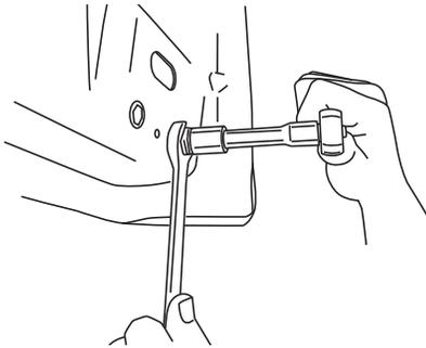
**WARNING:** Rivet Nuts not properly collapsed will not hold securely to sheet metal.
