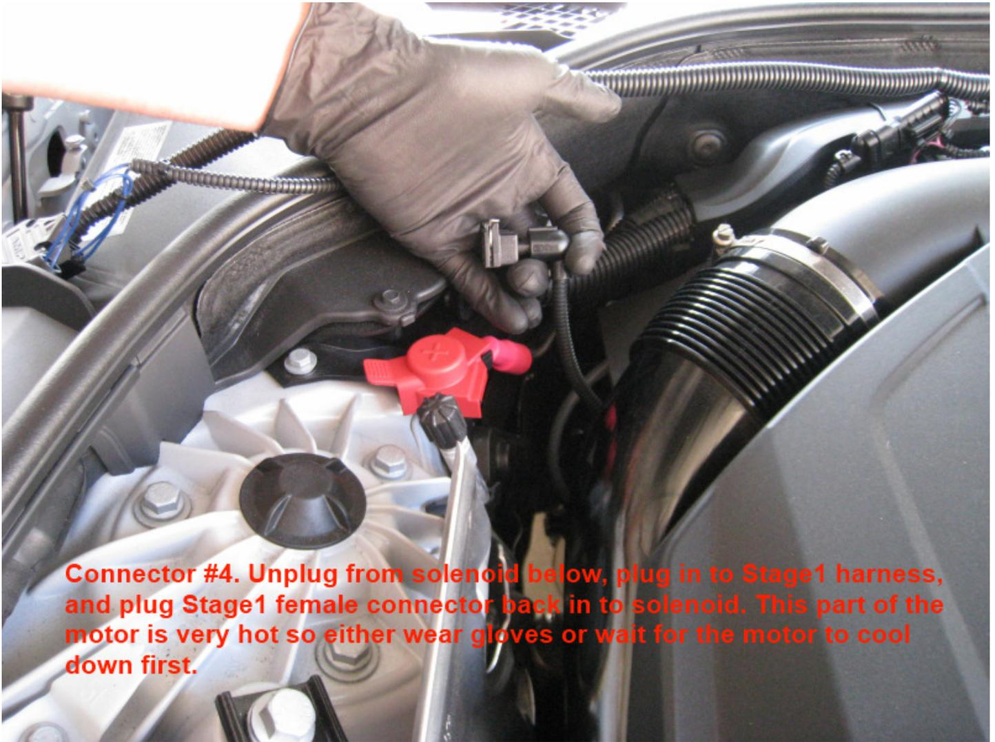
**Connector #4. Unplug from solenoid below, plug in to Stage1 harness, and plug Stage1 female connector back in to solenoid. This part of the motor is very hot so either wear gloves or wait for the motor to cool down first.**
