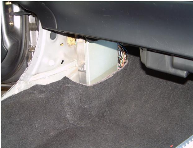
***Figure 1 – Passenger side kick panel showing ECU location***
