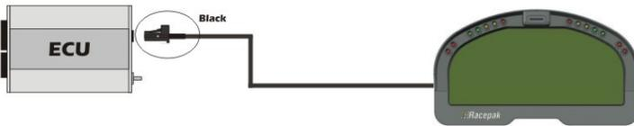
**Figure 9 – Haltech ECU connected to a Racepak Dash**
