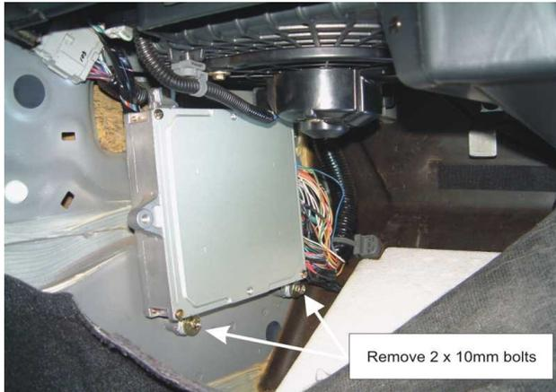
**Figure 2 – Factory ECU removal**
