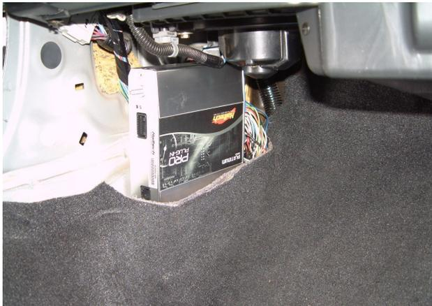
**Figure 3 – Haltech ECU Mounted to Factory ECU location**
