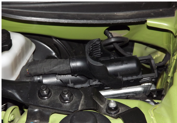
Figure 2 – Factory ECU disconnected and removed
