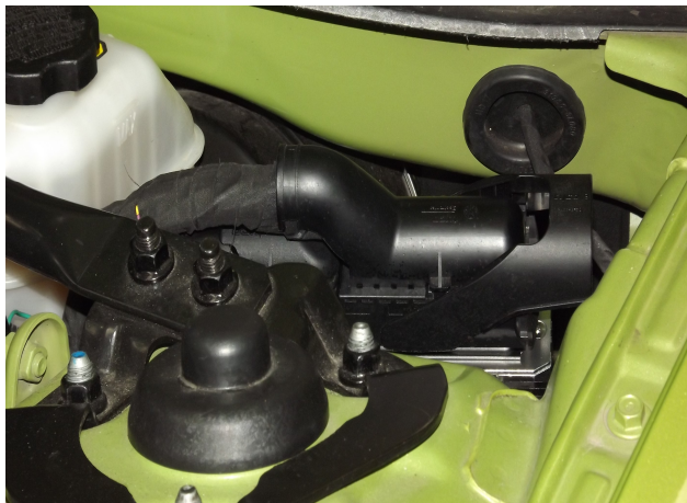
Figure 6 – Haltech Pro Plug-in ECU installed
