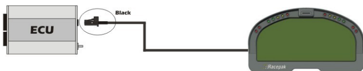
Figure 15– Haltech ECU connected to a Racepak Dash
