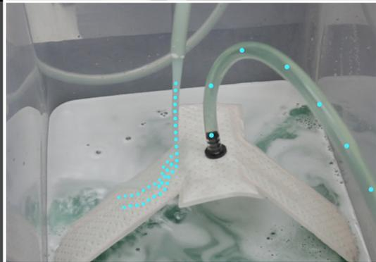
The sheer size and coverage area of the HydraMat allows it to pull fuel from virtually any area in the tank or cell eliminating the need for specialty reservoirs and pick up pumps saving cost and greatly reducing complexity.
