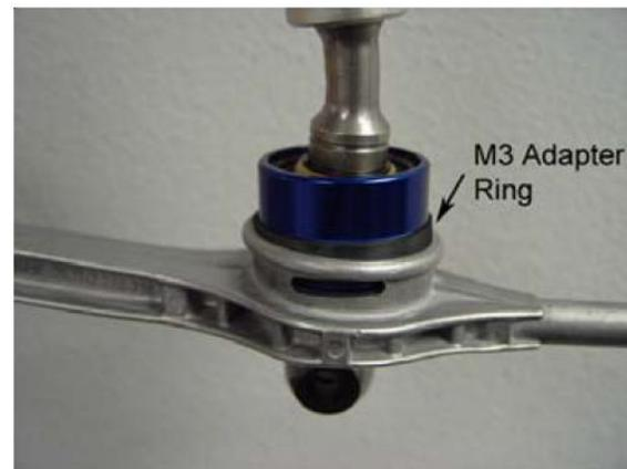
8. Thoroughly clean the inner portion of the gear selector arm housing. Using the supplied lithium grease, generously lubricate this area and the O-rings on the blue shifter pivot extension of the Dinan shifter.
