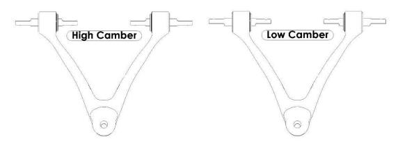
The upper Spherical bearings which feature a pin have the added feature of some camber adjustment. There are two settings as shown above. The Low Camber setting is typical for street use while the High Camber setting is typical in racing.
