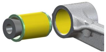
Apply a film of adhesive to both the control arm bore and bearing housing as shown above. Insert the bearing into the bore while rotating to ensure good coverage of the adhesive. Install the snap ring in the groove. The snap rings are installed by first starting the one end of the ring into the groove and working around the ring until the other end is seated.
