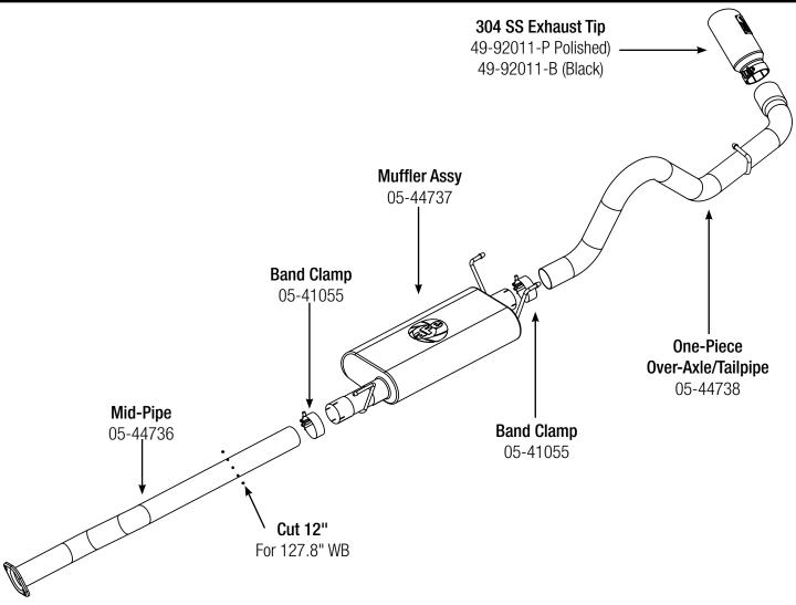
**Step 1: (Read Instructions prior to installation)** Remove your stock exhaust up to the catalytic converter from the rear of your truck working your way forward. Take caution not to damage the factory hardware and isolation mounts as they will be reused.
