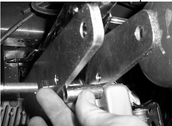
16) Secure the spacer between the brackets using a 10mm x 70mm bolt and 10mm lock nut.
