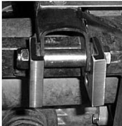
13) Next attach the top of the shock to the rear lift brackets using another 12 x 80 hex bolt and 12mm lock nut. (Use 1 left and 1 right bracket)
