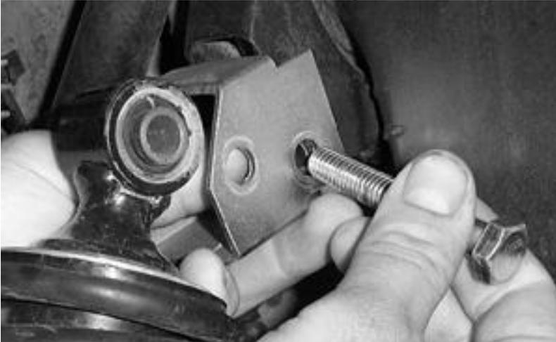
6. Next, insert the shock into the bottom of the tube bracket.
