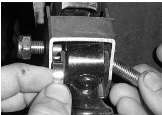
8. Fasten using the 10 x 55 bolts and 10mm nuts provided in the kit.
