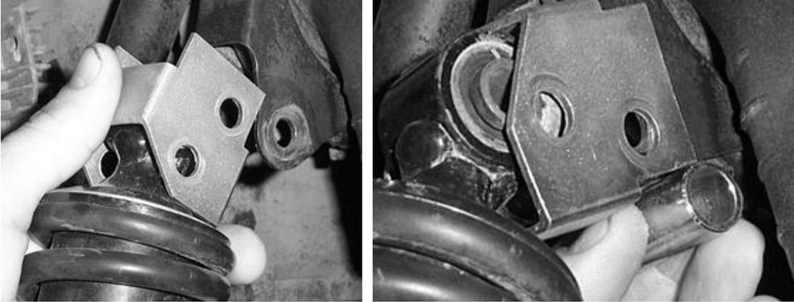
5. Secure the bracket to the ATV using the 10 x 55 hex bolts and 10mm nuts.
