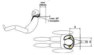
For Wrap Around installation of 3" webbing. Reduce results if using HANS specific 2"/3" webbing by 1"
