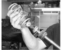
5. Reinstall the center spring collar and spring. Compress the spring and reattach the spring retaining collar.
