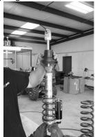
4. Install the new helper spring onto the shock.
