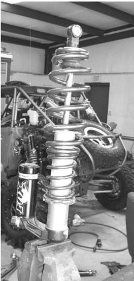
4. Compress the spring and remove the retaining collar from the shock.
