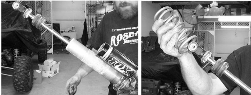
7. Reinstall the center spring collar and spring. Compress the spring and reattach the spring retaining collar.
