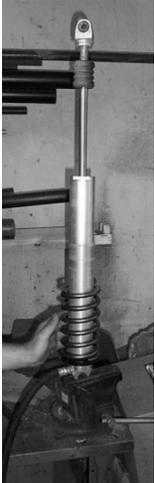
7. Reinstall the center spring collar and spring. Compress the spring and reattach the spring retaining collar.
