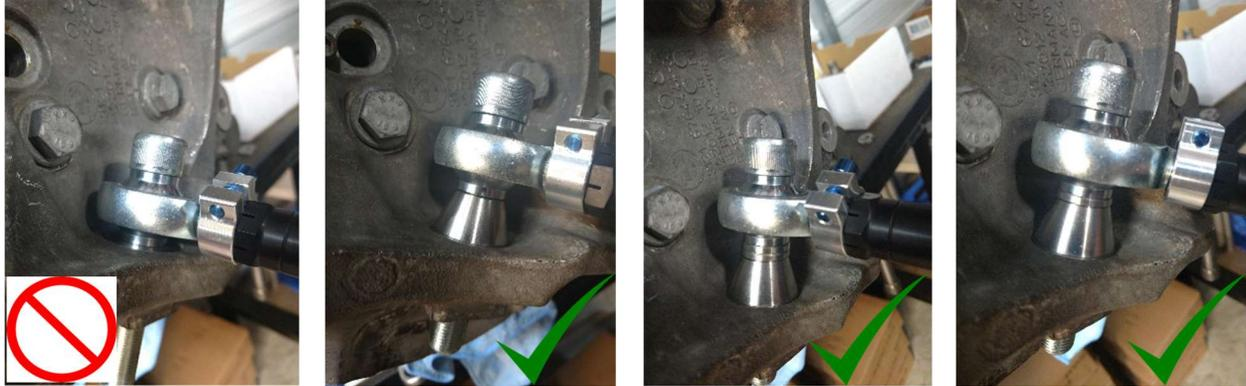
5. The shank (11) is a ½ inch Allen head. Tighten the nut at the top to **110 ft-lbs**. (Make sure to lubricate the threads; motor oil is fine.) Once tight, check for binding or any problems by moving the suspension through its full travel and moving the wheel lock to lock while doing so. Ensure that the spherical bearing does not bind (the edge of the ball bearing hitting or close to hitting the housing) under any of the above situations and there is no interference between suspension arms.
