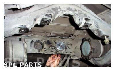
Install aluminum bushings with flat side facing towards front of car. Bushings are designed to be a press fit.
