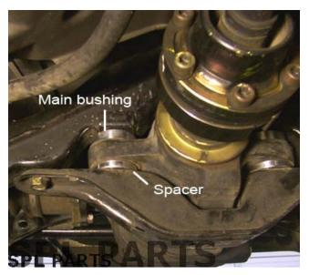
Knock out the OEM differential bushings on the front "ears" of the differential housing. Install the new aluminum bushings on the diff housing.
