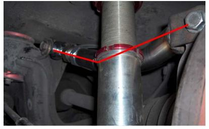
There is a small angle designed into the arm to allow it more clearance to the frame rail for lowered cars. If installed in the wrong orientation there will be LESS clearance to the frame rail than normal, and can result in damage or failure of the rear upper arms. Properly installed, the angle would be as shown
