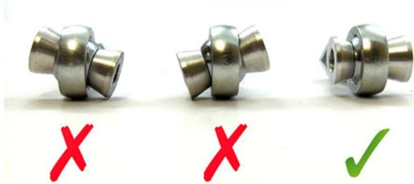
Make sure to keep the rod end bearing centered during and after an alignment. The far-right image with the green check mark is the correct position.
