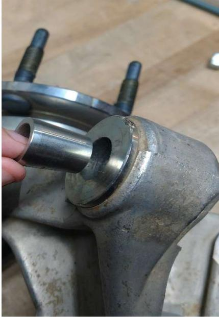
5. Place the tapered spacer inside the knuckle, then place the necessary roll center adjustment spacers for your application (the lower your vehicle, the more spacers you need).
