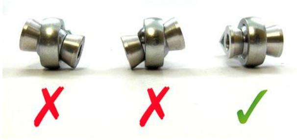
4. Once installed, ensure that both of the FK Rod Ends (4, 8) are centered and have full articulation. Lock them in place by tightening the Blue Titanium Socket Head Cap Screws (5) with a 3/16 allen wrench until the assembly does not rotate, to a maximum of **150 IN. lbs.**
