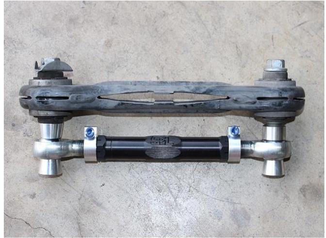
3. Install the SPL Parts Arm using the OEM hardware. Tighten the bolts to **74 ft. lbs.** (100 N/M) at both ends. **DO NOT OVERTORQUE.** *SPL Parts is not liable for any issues due to overtorque.*
