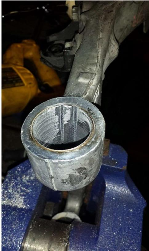
The sleeve can be removed once it has been cut all the way through in two locations lengthwise by prying the cut piece out with a narrow flathead screwdriver first, then collapsing the sleeve in on itself. After removal, carefully check the arm for and damage.
