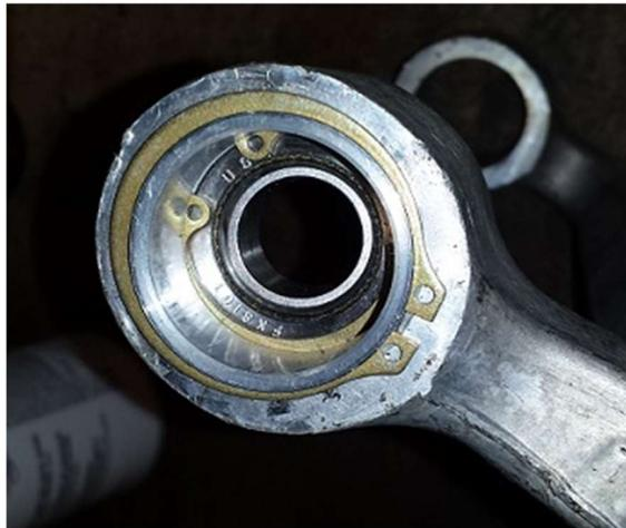
Once the bushings are installed with the lip flush against the arm, install the retaining clip on the other end to hold the bushing in place. Verify the bushings are secure, and install the solid spacers, then reinstall the arms on the car.
