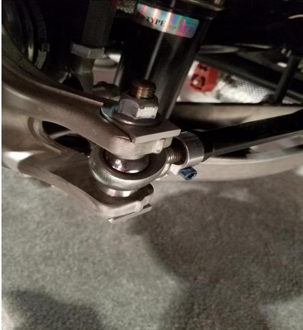
3. Install the Arm using OEM hardware at knuckle and the provided nut (18mm) and bolt (19mm) at the subframe and tighten them to 74 **ft. lbs.** (100 N/M). **DO NOT OVERTORQUE!** *SPL Parts is not liable for any issues due to overtorque.*
