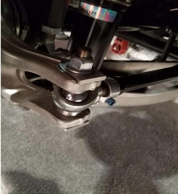
3. Install the Arm using OEM hardware at knuckle and the provided nut (18mm) and bolt (19mm) at the subframe and tighten them to **73.7 ft. lbs.** (100 N/M). **DO NOT OVERTORQUE!** *SPL Parts is not liable for any issues due to overtorque.*
