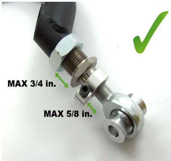
The next picture shows a properly threaded adjuster. The rod end (heim joint) will thread out about 2/3 the length of the adjuster. The maximum adjustment limits are shown in the picture.
