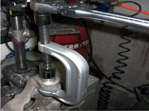
Press out stock bushing using appropriate bushing press and driver.
