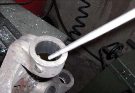
If the side of the knuckle which the new bushing goes in is not chamfered, use a round file to break the edge.
