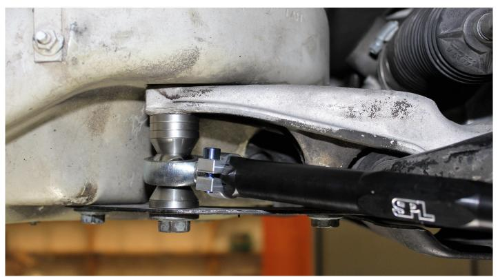
The picture above illustrates washers being used on the caster arm to account for anti dive on the front of the car by lowering the pivot point of the arm shown. Anti squat at the rear of the car is the same priciple, except the spacers are placed below the pivot point of the arm for anti squat.
