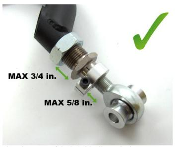
The advantage of the hybrid adjuster is that you can easily keep the rod end bearing centered during and after alignment. Make sure to keep the bearing centered as shown.
