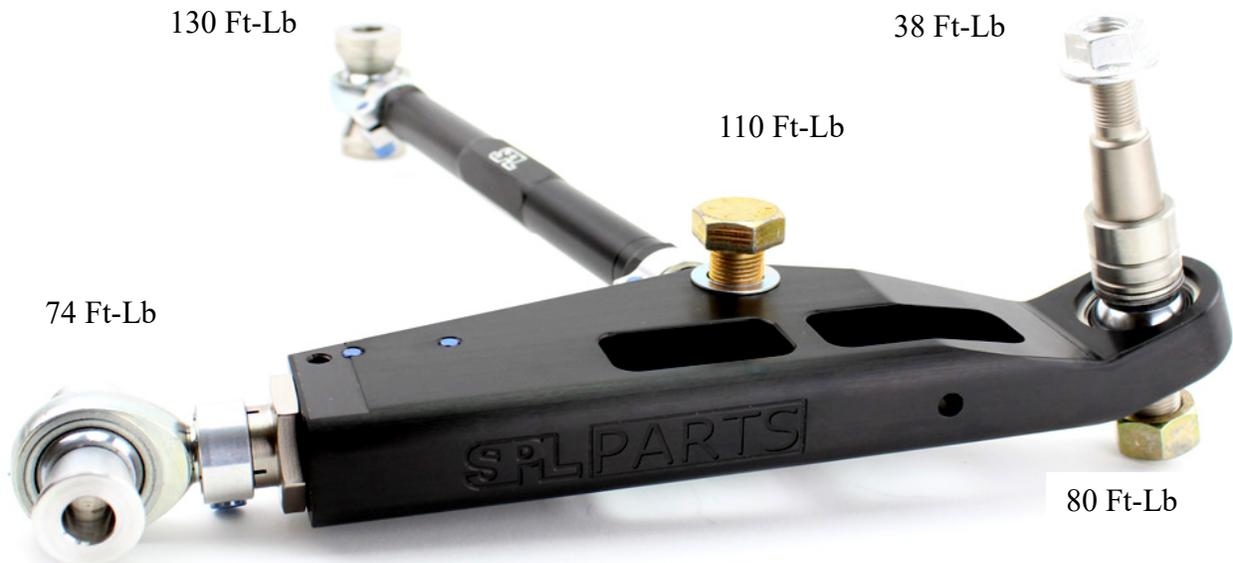
The picture above lists the torque specs. **DO NOT OVERTORQUE!** \*SPL Parts is not liable for any issues due to overtorque.\*
