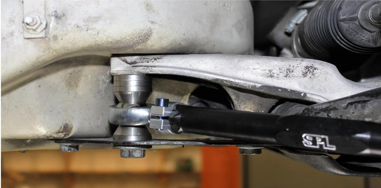
The picture above illustrates washers being used on the caster arm to account for anti dive on the front of the car by lowering the pivot point of the arm shown. Anti squat at the rear of the car is the same principle, except the spacers are placed below the pivot point of the arm for anti squat.
