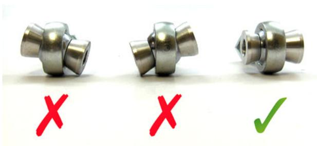
The advantage of the hybrid adjuster is that you can easily keep the rod end bearing centered during and after alignment. Make sure to keep the bearing centered as shown.
