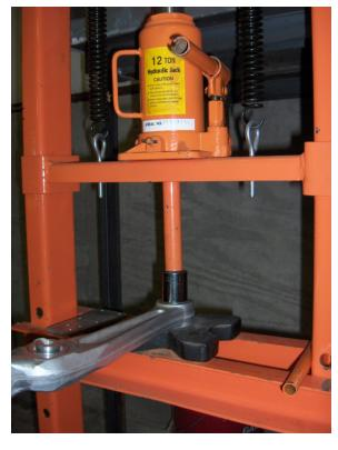
Using a hammer, lightly start the bushing into the bore, making sure bushing is square with the bore. Use press to continue pressing new bushing into compression rod.
