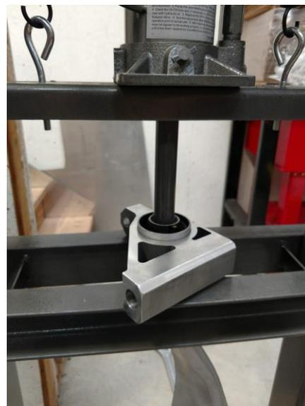
4. Once pressed out, clean the bore of any debris or scoring.
