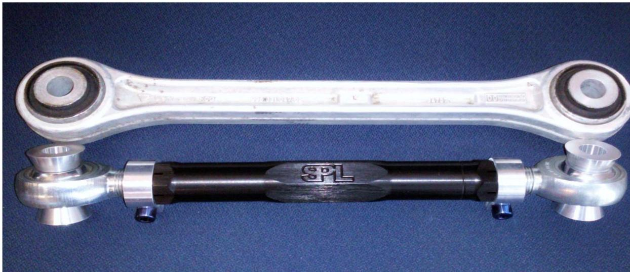
*Try to match length of new link to that of old, center to center of the bores.*
