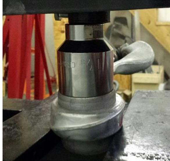
Be sure to have the arm level so the driver/socket can press out the bushing straight to avoid binding. Once square, press out the old bushing. Clean the bore of the arm, and smooth any nicks or burrs. The same socket can then be used to drive in the new bushing. Again, make sure to align the driver and bushing to go in straight and not bind.
