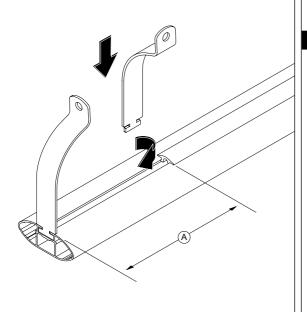
Cut the rubber buffer strip as shown, (B) = 110mm (for 4" conduit) and 160mm (for 6" conduit). Angle the pipe clamps back to allow room for the conduit. Place the rubber strip in between the clamps. Repeat steps 1 & 2 for the second set of clamps. Make sure the clamps are parallel to each other.
