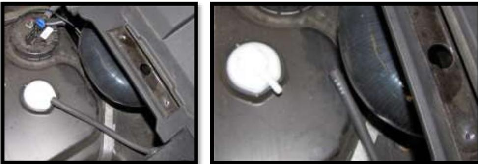
67. Insert the 5' vinyl hose **SK-VT-2** into the barbed fitting on the gas tank. You will need to route it up the cab. Drilling a routing hole in the plastic is optional. It just needs to be clear from being pinched or damaged.
