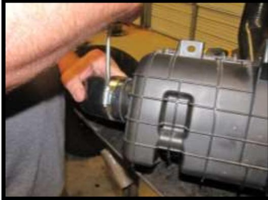
41. Reinstall the factory air box with the new air intake hose. The high lifter logo should be at the top of the hose and facing away from the cab.
