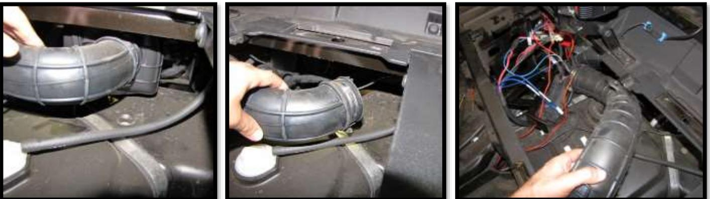
7. Next, loosen and remove the factory clutch intake hose. Also remove the adapter from the mouth of the clutch intake port fitting.
