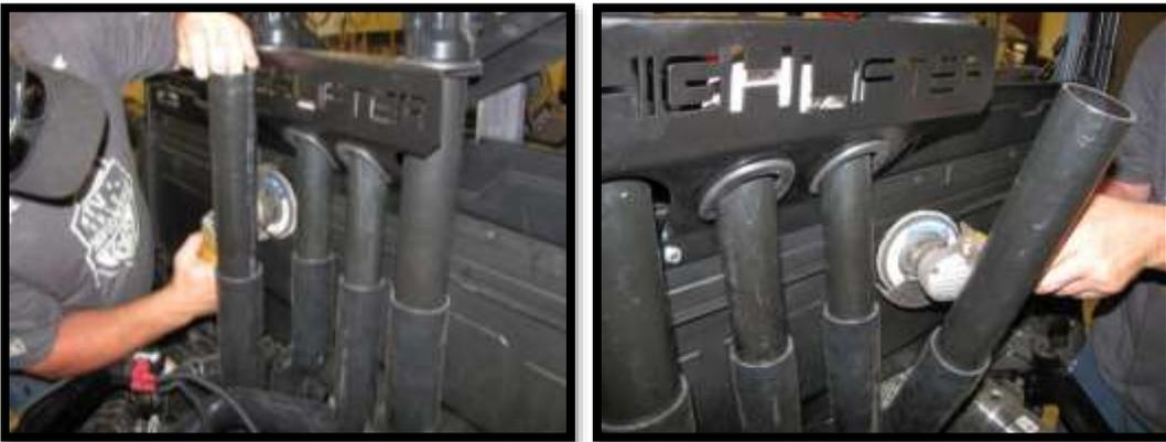
51. Slide the risers back into the riser plate. Then loosely attach the two **43R** riser caps to the top of the risers so that they sit flush to the riser plate. Do not fasten the hoses yet with clamps, you may need to make more adjustments in the following steps.
