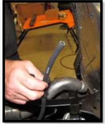
62. Insert a barbed fitting **BHF-14-ST** into the vent hose, followed by a bellow **VB01**. Use **11" zip ties** to secure the hose and bellow to the frame in a place it won't get damaged.
