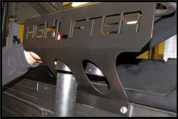
60. Once all final adjustments have been made. You need to attach and tighten the remaining hose clamps to the risers. Use a **HC40** for each 2" riser and a **HC36** for each 1 ½" riser.
