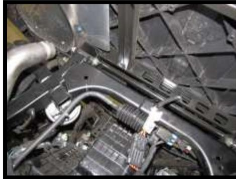
63. Find the front differential vent hose running up the frame on the front passenger side and disconnect it from frame. You will need the extra slack to reroute it up to the front storage compartment.
