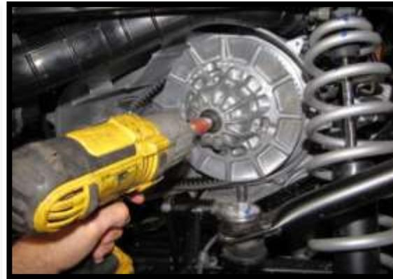
32. Before reinstalling the clutch housing cover, it needs to be sealed. Apply a generous amount of silicone to the clutch housing cover where it makes contact and seals to the housing.
