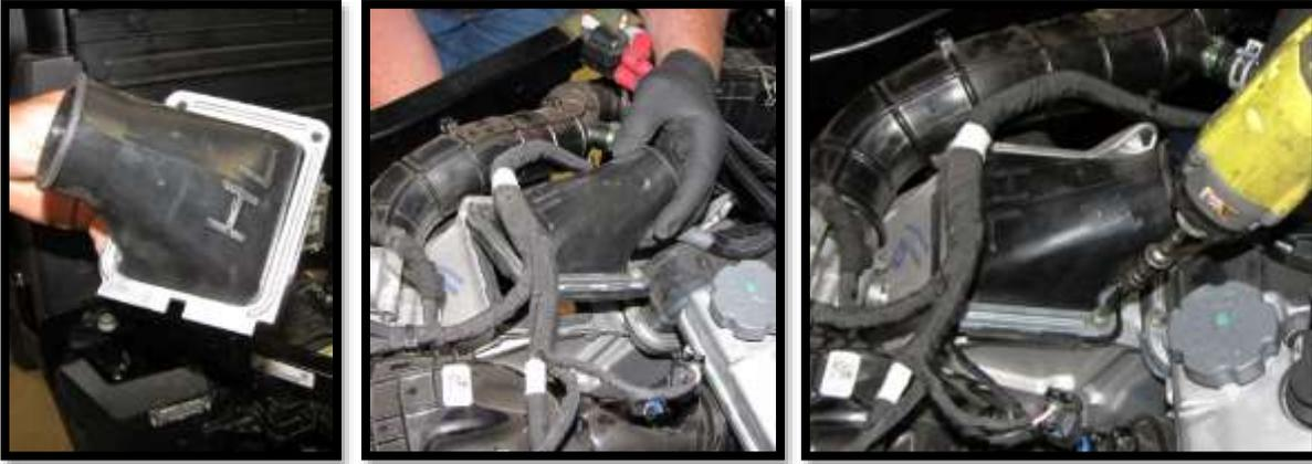
24. Apply a generous amount of silicone under and around the edges of the port inside the clutch housing. This will help ensure no water will leak in.
