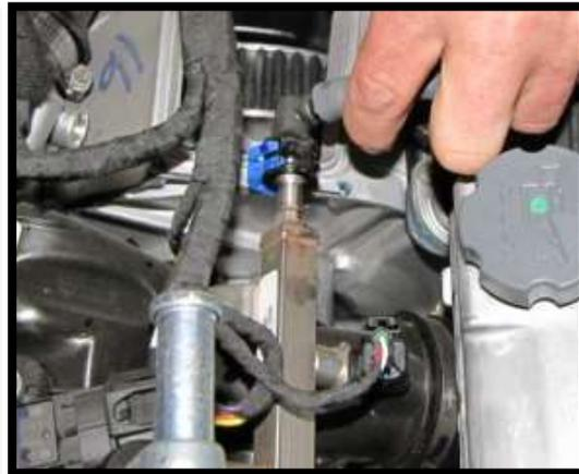
26. Remove the factory clutch housing inlet duct.
