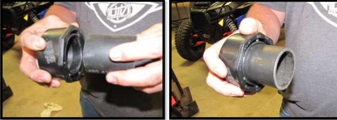
38. Insert the bushing adapter into the factory clutch intake hose and tighten the factory hose clamp.
