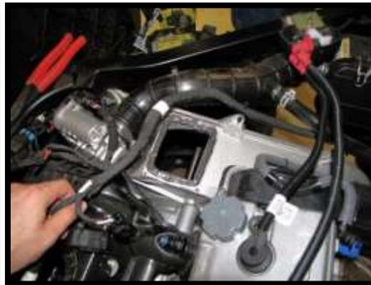
23. Slide the factory metal mount bracket onto the new **75N** clutch outlet duct. While installing, be careful not to pull the sides of the duct in. **This is necessary to prevent it from having an improper seal.** Once fastened, you will need to reach into the housing with your fingers and check for leaks or pulling of the edges.
