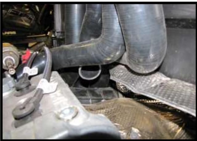
49. Loosely insert two **SK-P-223** (2 x 13 1/2" pipes) into the riser plate. You need to align them up so you can determine where to trim the plastic lip on the back of the cab in the next step.
