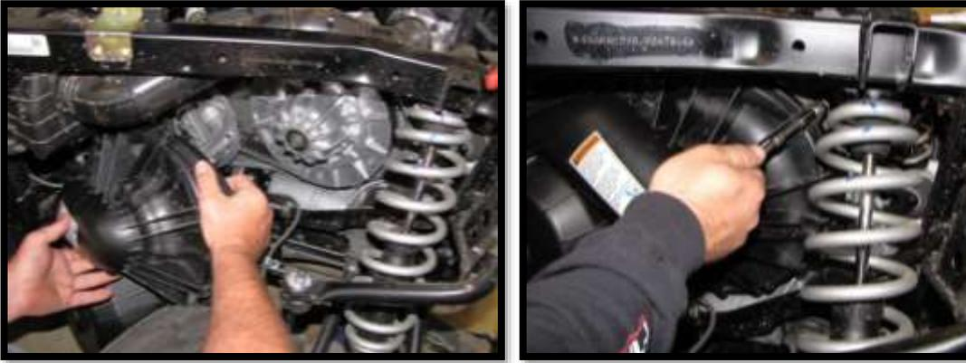
34. Insert two **27A** rubber grommets into the top holes of riser plate **75G**.
