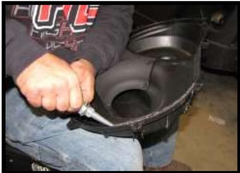
33. Reinstall the clutch housing cover and make sure it's properly sealed.
