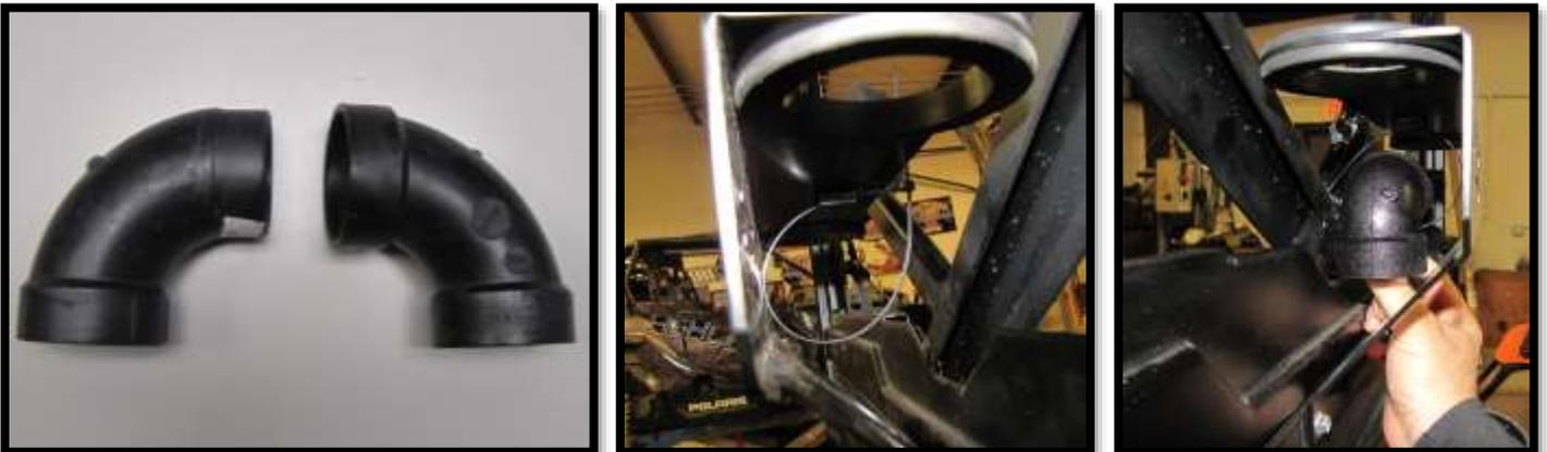
47. Slide two **SK-P-1527** (1 ½" x 10 ½" pipes) into the elbows. Then loosely slide the **RIGHT** riser into the corresponding clutch exhaust hose. Do not glue these into the elbows yet.
