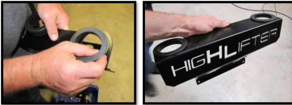
35. Next, you will install the riser plate using two **1 ½"** **self tapping screws** to the back of the cab. There are two indentions in the plastic you can use as guides to drill the screws into and keep the riser plate centered.
