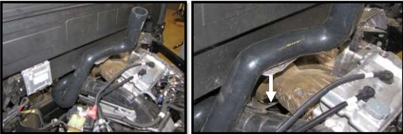
40. Next, slide the new air intake hose **75A** onto the air box inlet. Position it so that the high lifter logo is at the top of the hose and facing away from the cab when you reinstall the air box in the next step. Doing this before installing the air box will make the installation much easier and prevent having to adjust it. Attach and tighten down with hose clamp **HC40**.
