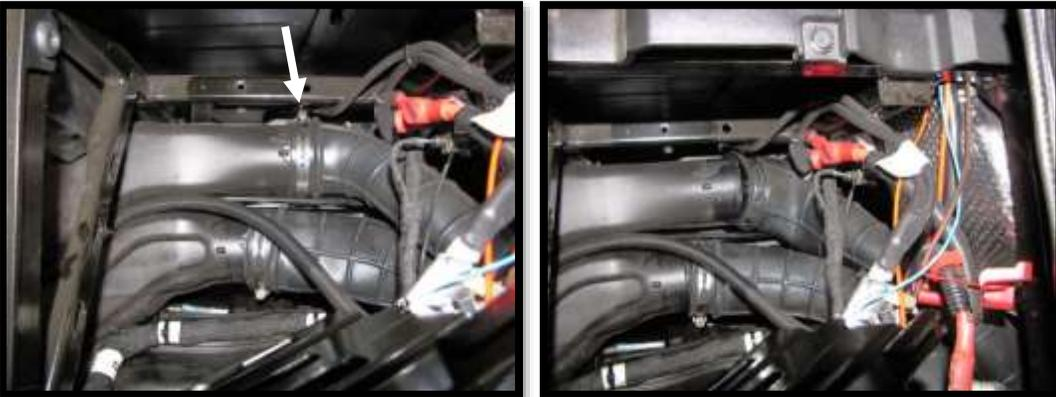
6. Now loosen the clamp from the air box inlet, and remove the factory air intake hose.
