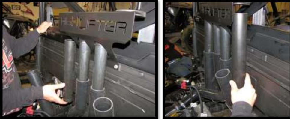
50. Once the 2" risers are lined up and you know where to trim, slide them out of the riser plate and pull them back. Use a grinder to trim the plastic lip so that each 2" riser can sit flush to the back of the cab.
