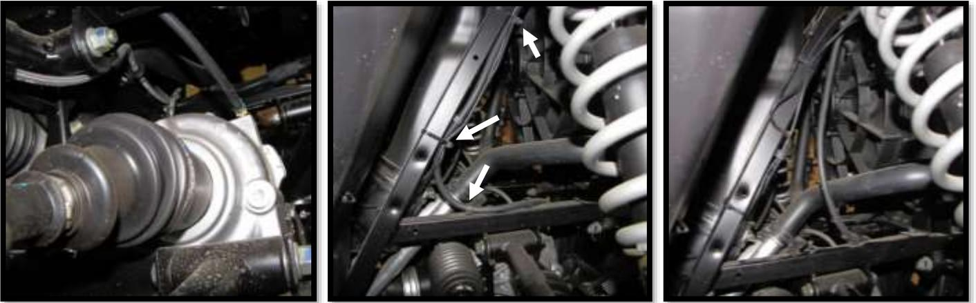
64. Find any precut holes or opening to route the vent line through to the front storage compartment. Once through, insert a barbed fitting **BHF-14-ST** into the vent hose, followed by a bellow **VB01**. Use **11"** zip ties to secure the hose and bellow in a place it won't get damaged.
