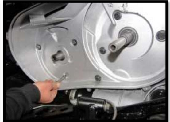
16. In the next steps, you will remove the four bolts from the right side of the clutch housing.
