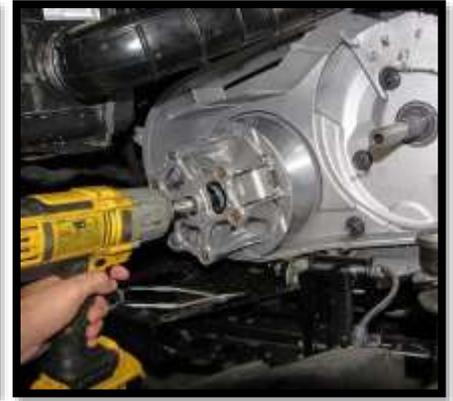
31. Reinstall the belt and secondary clutch
