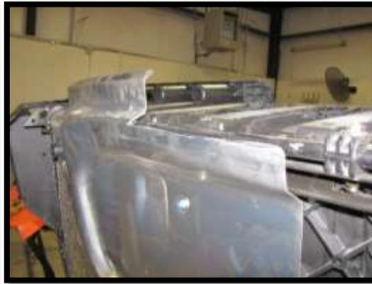
55. Find the bed plate **75L**. Center it on the bed using the large holes and where it meets the snorkels. Then trace the inside with a marker.
