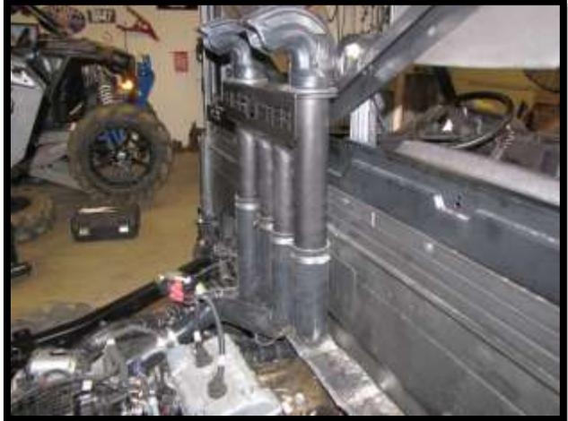
71. Reattach the lift support strut to the bed and close the bed. Check fitment, clearance, and make any necessary adjustments.
