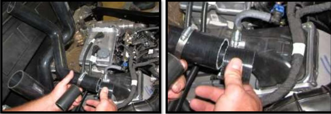
45. Next, slide the **SK-P-1506** (3" pipe) into the clutch outlet duct. Center it and slide the clutch exhaust hose on. Attach and tighten with two **HC36** hose clamps.
