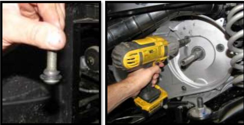
19. Before you can install the new clutch outlet duct, you will have to remove the fuel rail. Removing it will allow clearance so you can install it.
