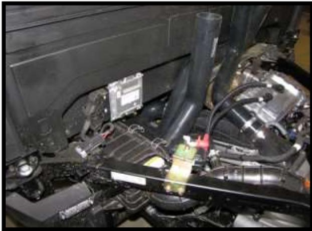
42. In the following steps you will install the new clutch exhaust hose to the clutch outlet duct.
