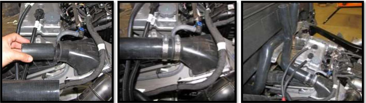
46. Connect and glue the 90 degree elbows **SK-EL-1501** and **SK-EL-1502** together. Then secure the elbows underneath the top of the riser plate with a heavy duty **18"** zip tie so that they are snug. This will keep them in place while you line up the risers in the next steps.
