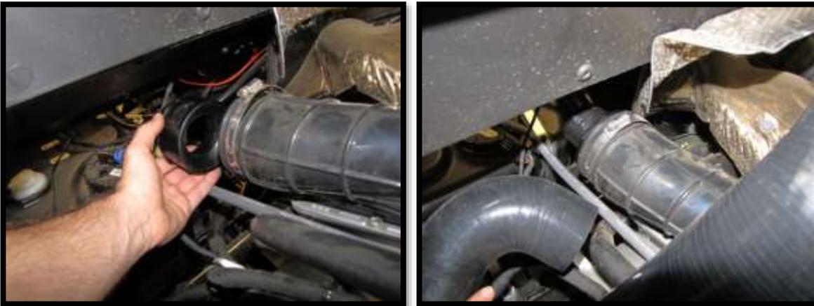
39. Insert the new clutch intake hose **75B** onto the pipe. Align the hose to the back of the cab and riser plate in the proper position. The high lifter logo should be at the top of the hose and facing away from the cab. Attach and tighten it with hose clamp **HC40**. You may need to bend the exhaust heat shield down at the edge to provide more clearance for the hose.
