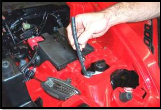
32. Drill a 1/2" hole in the base of the post.
