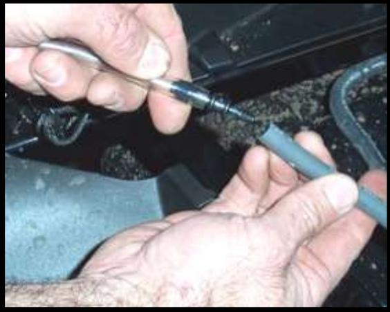
49. Route the vent line up the frame from behind the passenger seat up to the hole in the cage.
