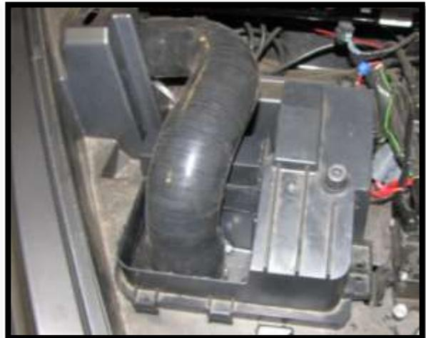
11. At the cup holder, pull the end of the hose out and slide hose clamp (**HC36**) on the end of the hose. Then slide a 2"x3.5" pipe (**SK-P-252**) half way into the hose and tighten the hose clamp.
