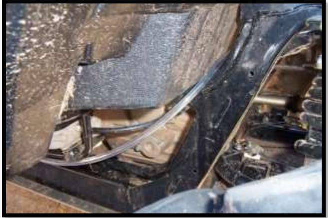
57. Secure the line along the way. Push the vent line up from under the UTV to an opening in the plastic nearest the hole you drilled for the rear differential. Insert the vent line into the hole as far as you can.
