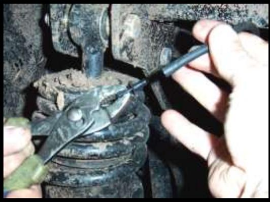
54. Insert into the rear differential vent line the remaining 1/4" x 3/16" reduction barb (**BHF-R-14316-ST**) provided in the kit.
