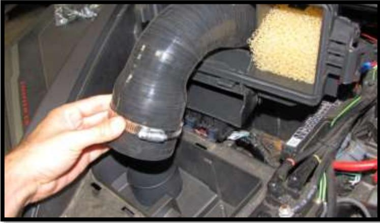
10. Slide the hose onto the intake inlet and tighten the hose clamp. Then slide down and secure the intake box back in place.
