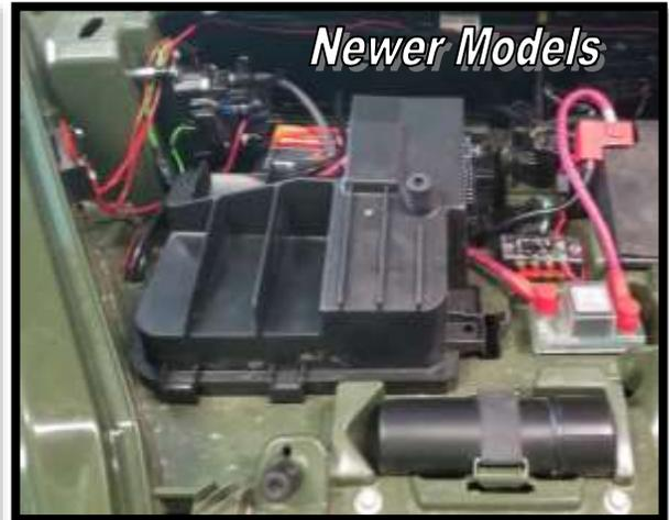
2. Remove the cover and foam intake filter.
