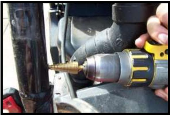
28. Next you will need to cut a 4ft section from the vent line (**SK-VT-1**) and run it through the fender near the base of the post. Similar to the way you routed the air intake hose.
