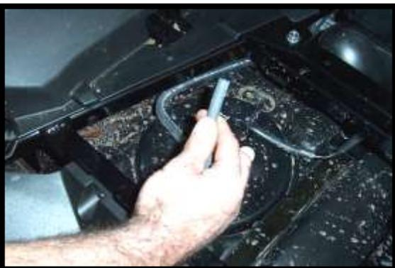
47. You will use another 5ft of clear 1/4" vent line (**SK-VT-1**) supplied in the kit to extend the gas tank vent line up to the hole you drilled in the cage.
