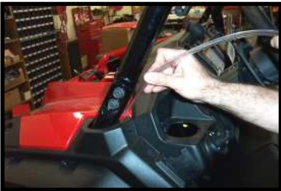
37. Insert the hose into the cage post, pushing it up the post until it stops. Pull any remaining slack back under the hood. Secure the loose line under the hood with the **11" zip ties** provided.
