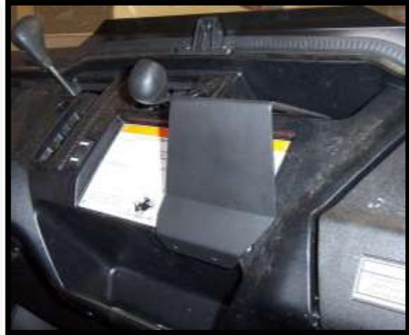
20. Using (4) (PTS1034P) screws, attach the bracket to the dash. Then reinstall the factory cup holder into the new bracket.
