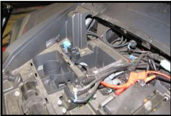
3. Remove the passenger cup holder from the passenger side of the UTV.
