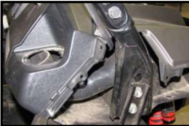
9. Slide the modified plastic cover onto the hose followed by hose clamp (**HC52**).
