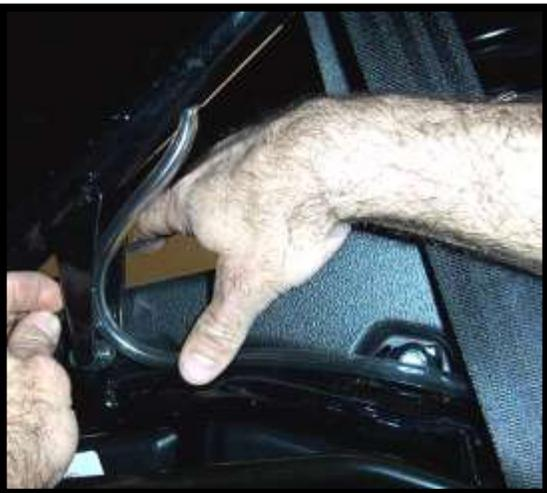
52. Locate the rear differential vent line. It is connected to the frame just above the differential. Follow the line from the differential if you can find where it is attached to the frame.
