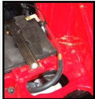
38. On the driver's side of the UTV you will need to drill (2) ½" holes in the cross member on the cage. Drill one lower on the cross member and one higher. The lower hole will be for the rear differential and the higher hole will be for the transmission vent line.
