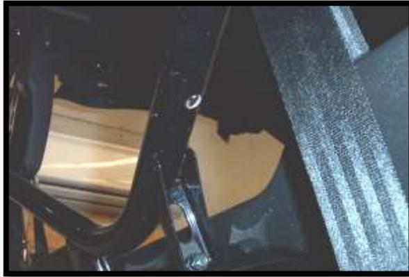
45. Located under the passenger seat is the gas tank and also where the gas tank vent line, vents into the frame.
