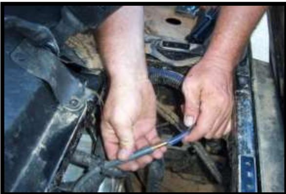
42. Route the vent line up through the plastic behind the seat to the hole drilled for the transmission vent line in the frame cross member. Insert the vent line into the hole as far as it will go.
