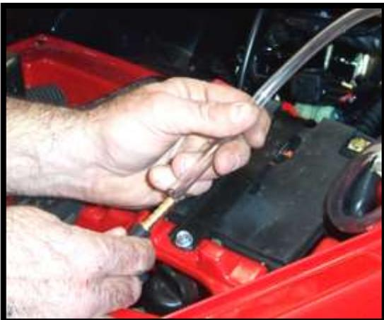
35. Inset the other end of the vent lineup from under the hood through to the hole near the cage post.
