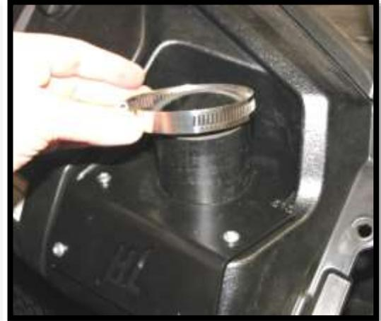
14. Find hose (78K). Insert it over the pipe and slide and through the clamp. Then tighten the hose clamp.
