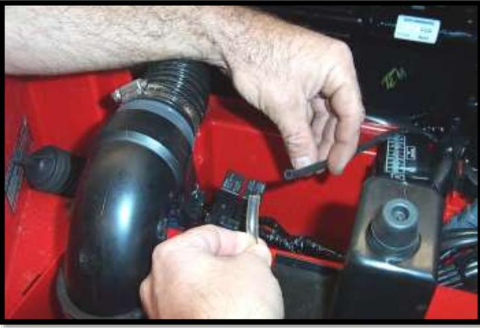
24. Included in the kit is a 1/4" x 3/16" tee (SK-BT-14316). You will need to connect the two lines to the tee.
