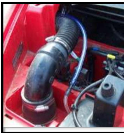
30. Insert the other end into the ½" hole you drilled into the post. Make sure to push the hose up the post as far as you can. Secure the line with (**11" zip ties**) provided.
