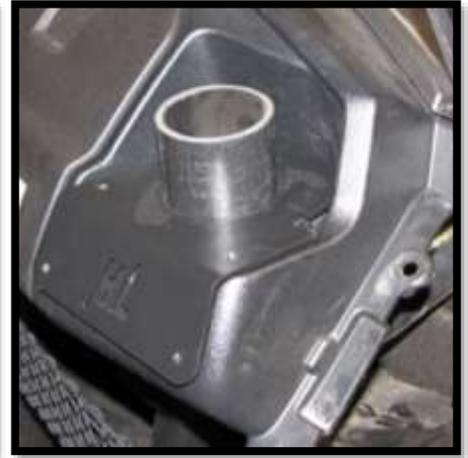
13. Secure the bracket with (5) (PTS1034P) screws. Then slide a hose clamp (HC36) over the pipe.
