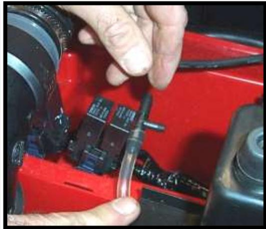
**NOTE:** It will help to heat up the vent line with a heat gun or hair dryer so to make it more pliable so it can fit in the barb.
