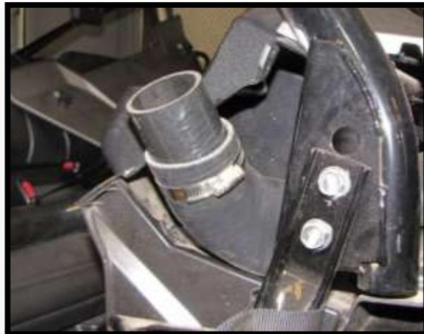
12. Insert the pipe and hose in the cup holder hole. Then slide bracket (80Q) onto the pipe.
