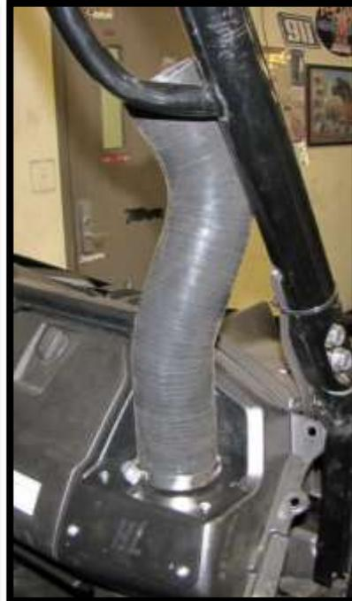
15. Insert the 2" x 16.5" pipe (SK-P-250) into the hose, followed by clamp (HC36).
