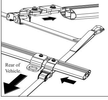
Wrap the snap hook end of the strap over the ladder runs. Snap the hook onto the hook bracket ensuring the safety latch is fully closed onto the hook. Pull the strap to tighten around the ladder runs. Check that the ladder is secure. To release the ladder, press the camlock latch and pull the strap back through the camlock, unhook the snap hook, if travelling with out a ladder, locate the snap hook onto the hook bracket.
