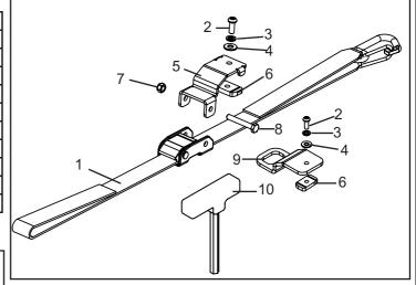
1 Remove the sportz leg if required. Slide the snap hook bracket and strap bracket into the end of the crossbar as per the diagrams. Position the camlock and hook bracket to suit the ladder, tighten the bolts with the allen key provided.
