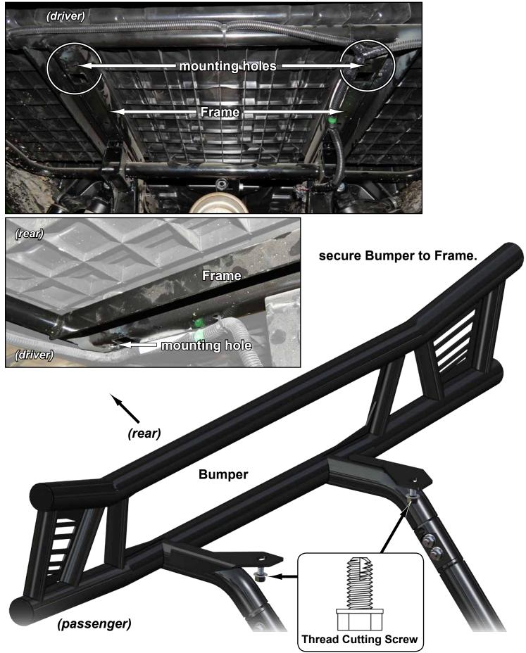
Align to machine and tighten hardware completely.
