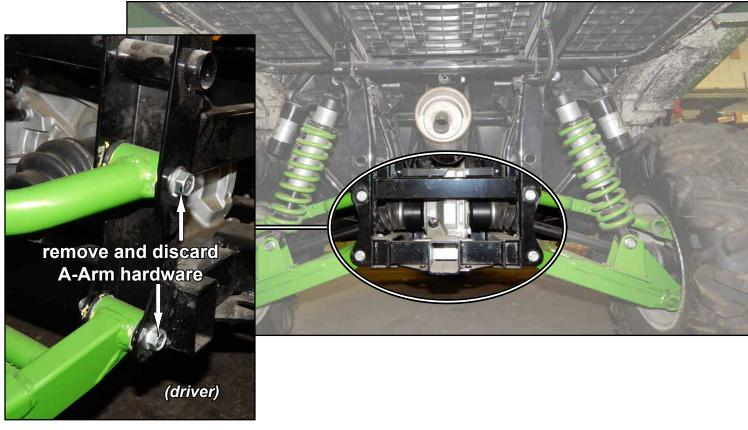
Do not tighten hardware completely unless noted.
