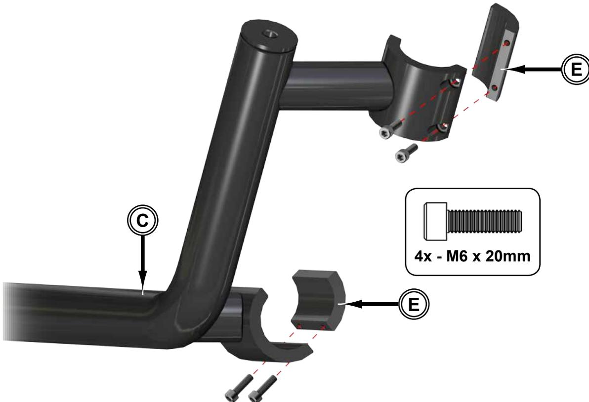
**Do not tighten hardware completely unless noted.**
