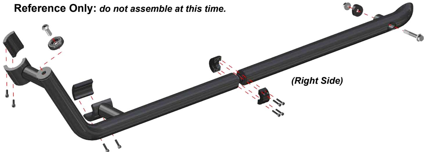
**Do not tighten hardware completely unless noted.**
