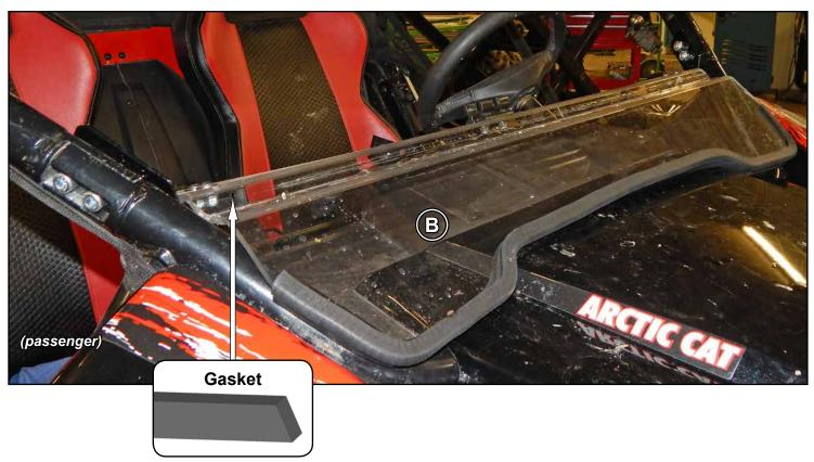
Install Gasket to this surface. Gasket to run length of Lower Windshield (B).
