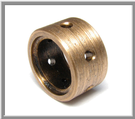
Figure 10: Journal Bearing Contaminated Oil Visible Scarring on Inner and Outer Diameters
