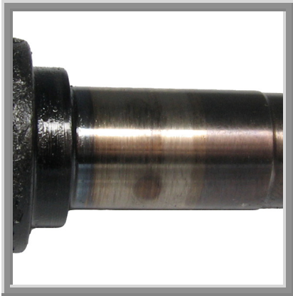
Figure 6: "Hot Shutdown" Turbine Wheel Shows Visible Bearing Pattern and Heat Discoloration
