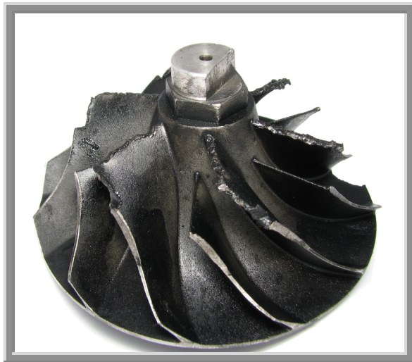
Figure 12: Compressor Wheel Foreign Material Severe Damage to the Vanes on the Wheel
