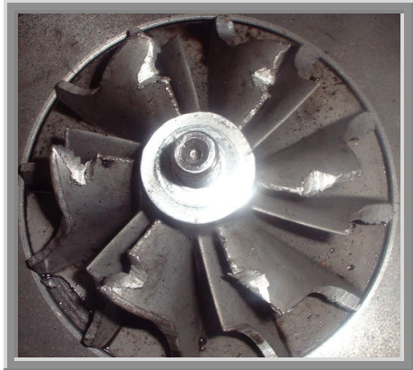
Figure 17: Compressor Wheel Lock Nut Failure Nut is missing, foreign object Damage to vanes
