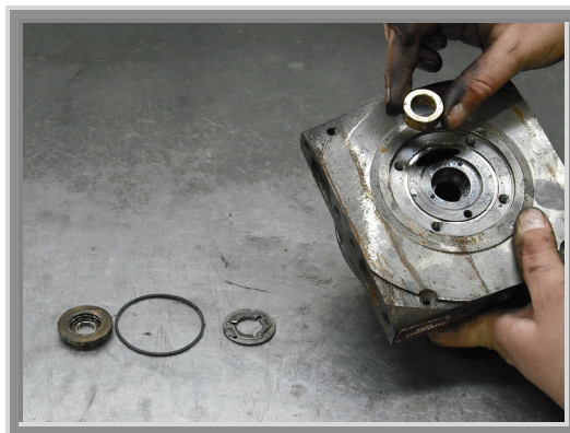
Figure 6: Remove Bearings, Washers, Etc.
