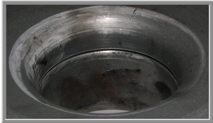
Figure 18: One Sided Wear on Compressor Housing Can be caused by improper manufacturing or assembly
