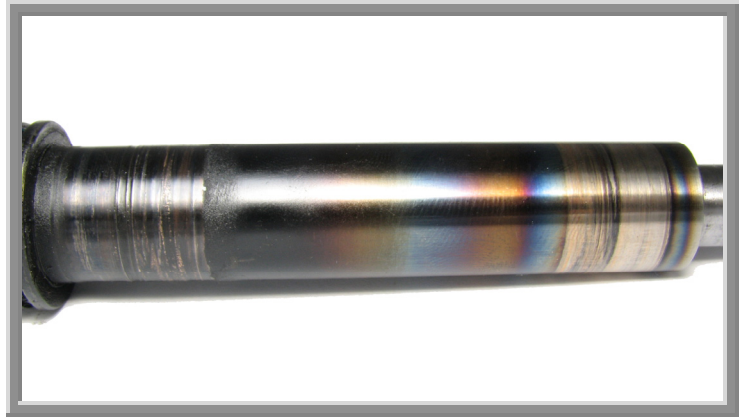
Figure 7: Turbine Shaft Lack of Lubrication Turbine Wheel Shows Visible Heat Discoloration and Smeared Wear
