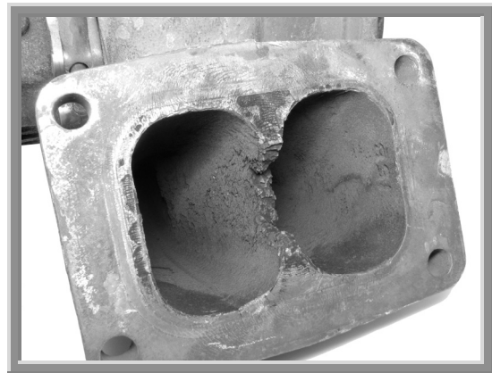
Figure 15: Turbine Housing High Exhaust Temp Erosion of Web Caused by High Temperatures
