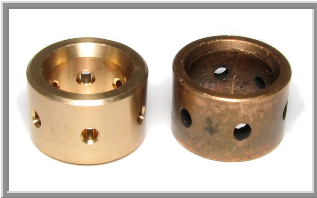
Figure 8: Journal Bearing Lack of Lubrication Left = New Bearing; Right = Smooth Wear & Heat Discoloration
