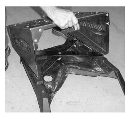
11. Use the ¼" x 1" bolts, ¼" washers, and ¼" lock nuts provided. Place a ¼" washer on the top in the bolt hole then insert the ¼" x 1" bolt through the washer and bolt hole. On the underside of the rack place a ¼" washer on the bolt and secure it using the ¼" lock nut.
