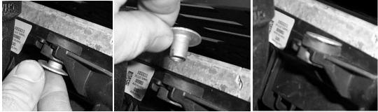
17. Attach the radiator to the kit. Insert the ¼ x 3 ½ carriage bolts through the top of the face plate. Place the two long spacers onto the bolts. Next place the radiator onto the bolts and spacers, then fasten the radiator with the ¼ flat washers and ¼ lock nuts.
